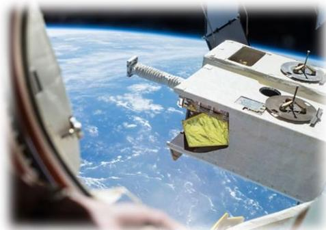
6. On-orbit Extraction: Dextre extracting Payload from Cargo Rack in Dragon Trunk.
